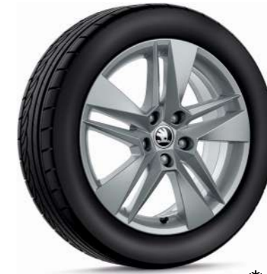
Markab light-alloy wheel 6.5J x 17" ET41 for 215/55 R17 3V0 071 497F 8Z8 | silver metallic ❄️
